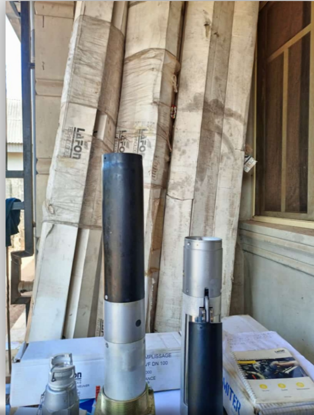
LAFON OVERFILL PREVENTION VALVE
